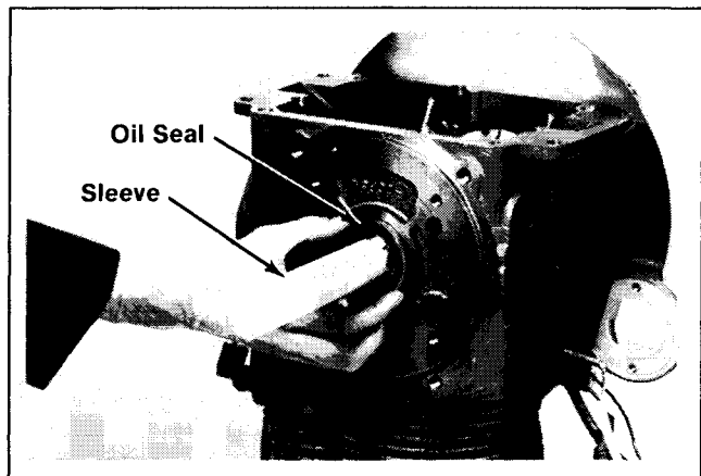
Figure 12-33. Installing Oil Seals Using Sleeves.
