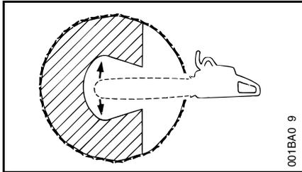
First, cut a large, wide felling notch. Make a plunge cut in the center of the notch.
