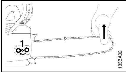
Retensioning during cutting work:
