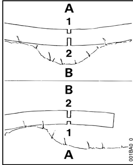
5. Logs under strain: Risk of pinching! Always start relieving cut (1) at compression side (A). Then make bucking cut (2) at tension side (B). If the saw pinches, stop the engine and remove it from the log.
