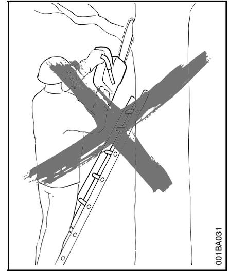
Never work on a ladder, or on any other insecure support. Never use the saw above shoulder height.
