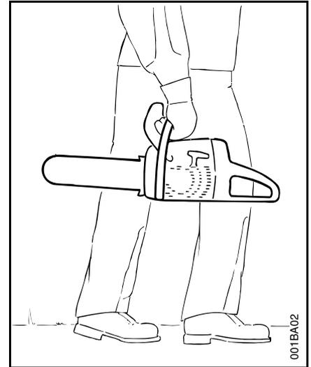
The chain guard (scabbard) should be over the chain and the guide bar, which should point backwards. When carrying your saw, the bar should be behind you.
